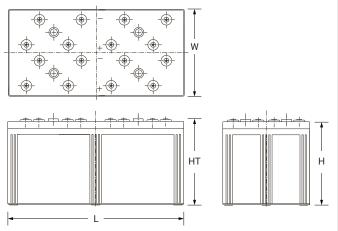
L: 27.91 (709) W: 13.77 (350) H: 13.26 (337) HT: 13.74 (349) Tolerances are +/- 0.04 in. (+/- 1mm) and +/- 0.08 in. (+/- 2mm) for height dimensions. All data subject to change without notice.
